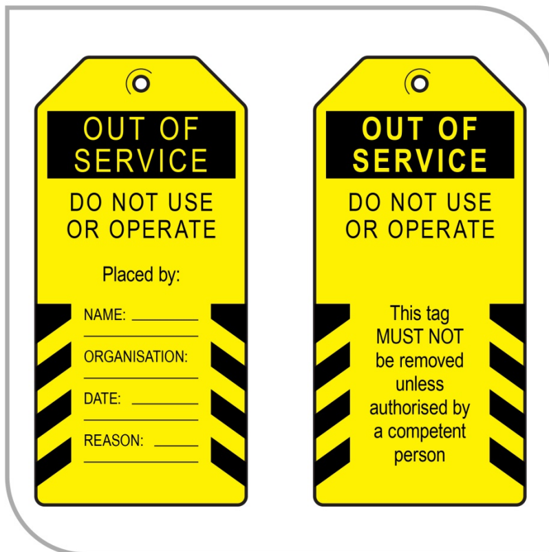
Figure 8: Example of an out-of-service tag
